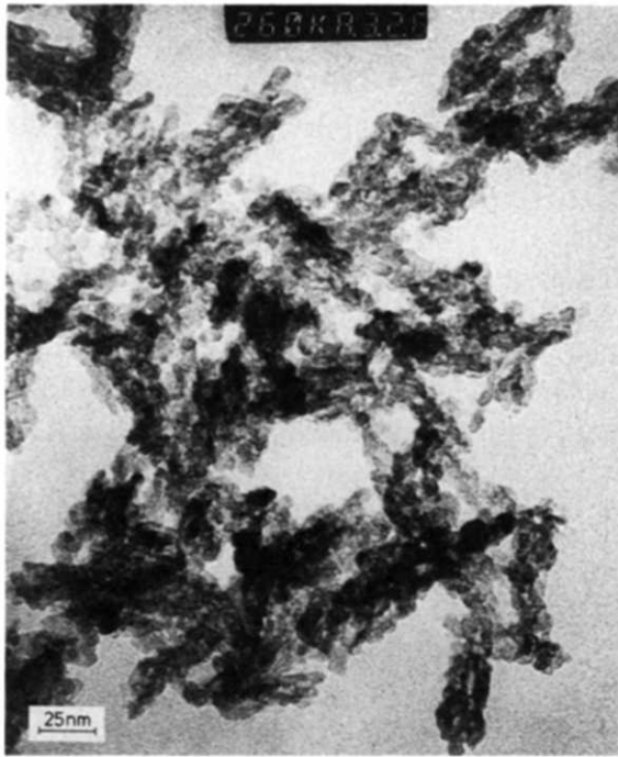
Fig. 9. Incompletely hydrothermally processed BaTi acetate gel; fibrous character of gel precursor is still preserved (TEM, 'nucleation of BaTiO 3 ').
